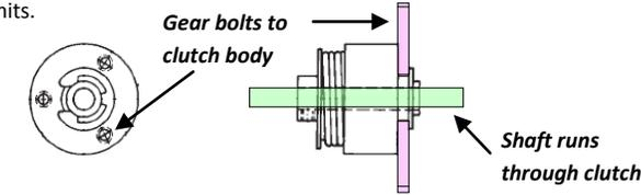
*Gear bolts to clutch body*
