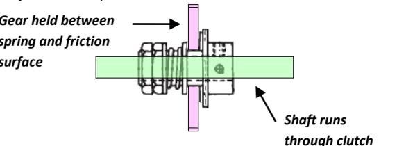
*Gear held between spring and friction surface*
