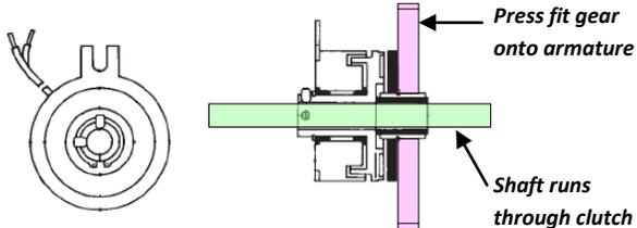
*Press fit gear onto armature*
